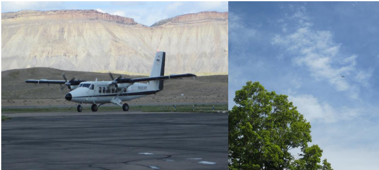
Figure 11: The instrument payload is installed in a DeHavilland DHC-6 Twin Otter shown on the left and data are collected at a nominal flying altitude of 1000 m above ground level as shown on the right
