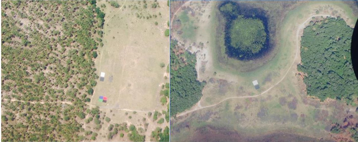
Figure 27: Radiometric calibration tarps as viewed from the aircraft on May 7 (left) and May 19, 2014 (right). Photos courtesy of NEON AOP
