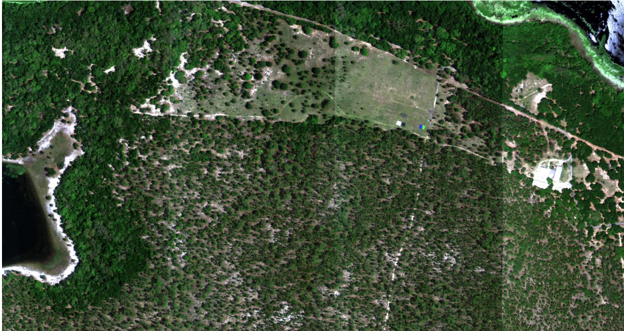
Figure 40: A true color image of a portion of the hyperspectral data showing several flight lines stitched together to form a mosaic for the entire site. Ground calibration tarps can be seen in the field
